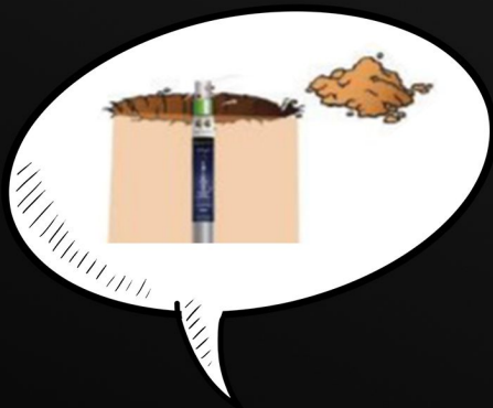
Step 3. Insert The Elec Power Earthing Electrode.
